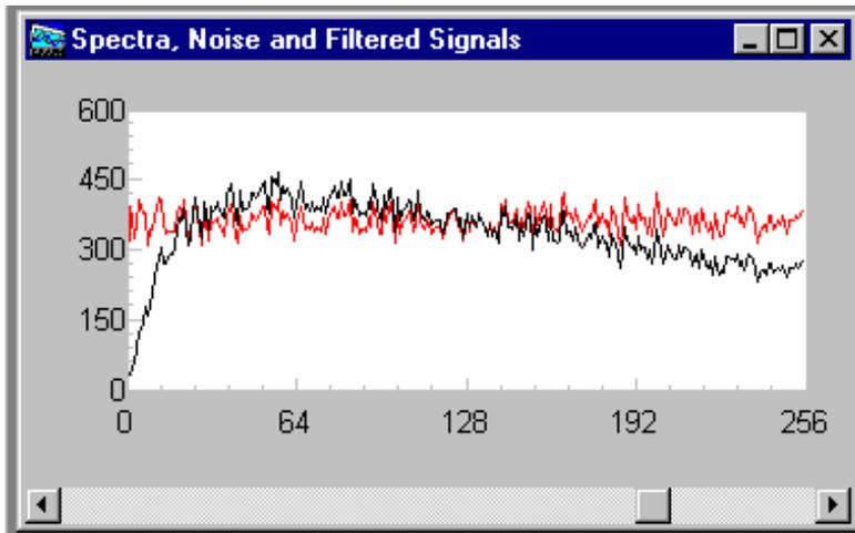
The two spectral plots are obtained by passing the pre-filter and post-filter data streams through FFT processing. The results of analyzing randomized data streams are very noisy, so groups of 64 spectra are averaged.
