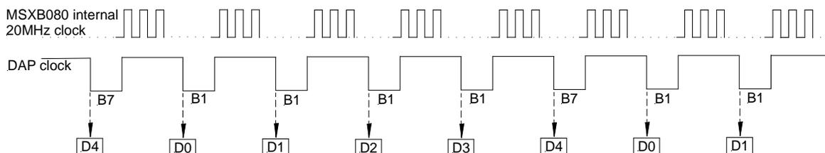
**Figure 9. Timing diagram for sampling one MSXB080 module**
