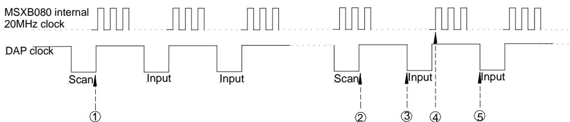
Figure 8. Timing diagram for scan and input addresses
