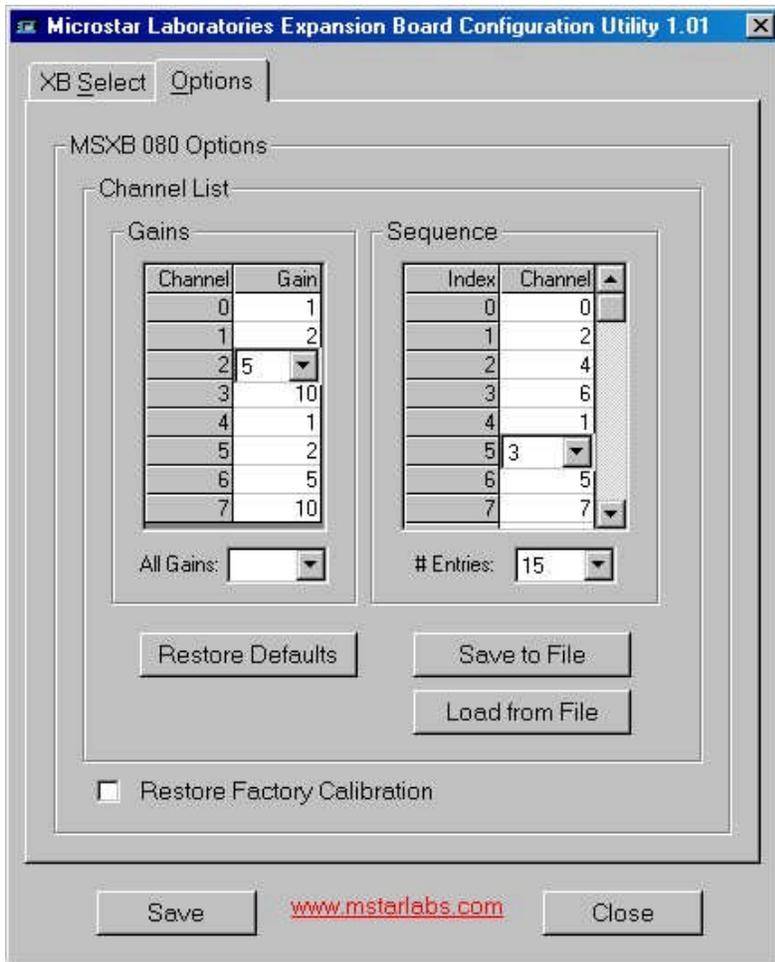
**Figure 7. Channel list of a MSXB080 module.**
