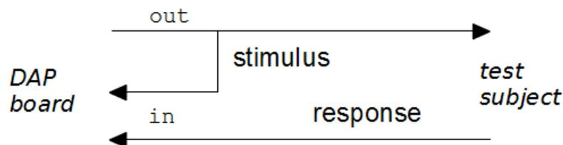
This loopback configuration, monitoring the output signal sent to the subject under test, and simultaneously monitoring the response, establishes a very tight time-association between the stimulus and response signals. There can be some delay before the hardware updating cycles begin signal output
