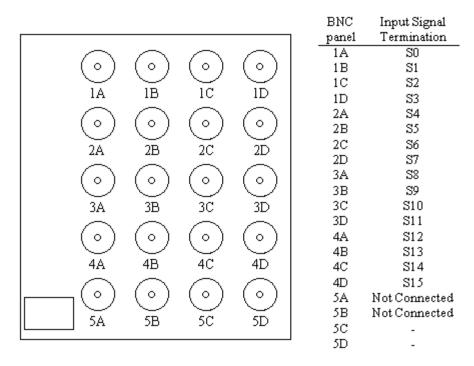
Each BNC panel occupies five slots in an industrial enclosure and it provides 20 isolated BNC connectors. Each BNC input connector has a black wire and a red wire. The red wire is connected to Sx, where x represents the input signal termination, whereas the black wire is connected to Gx. For example, the red and black wires of 1A should connect to S0 and G0 on the MSXB 037 board.
