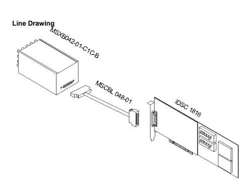
HwCfg05 Hardware Configuration with an iDSC Board
