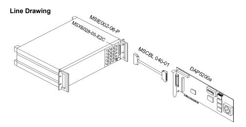
HwCfg04 Hardware Configuration with Simultaneous Sampling
