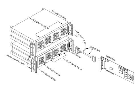
HwCfg02 Hardware Configuration with Input Expansion
