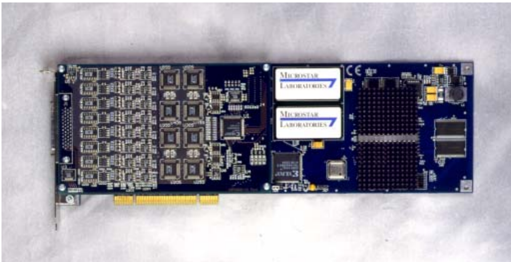
iDSC 1816: 1.2 million filtered samples per second
